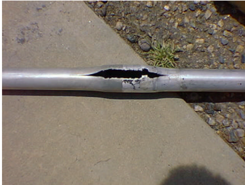
Figure 4.11. Longitudinal tearing of the tube in Test 3.
