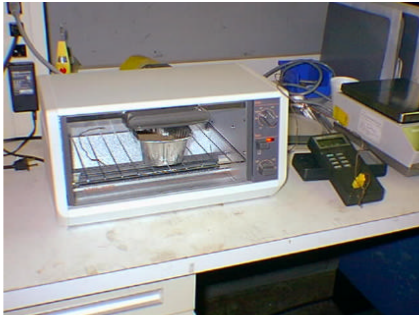
Figure C.4. Performing the soil moisture content analysis.
