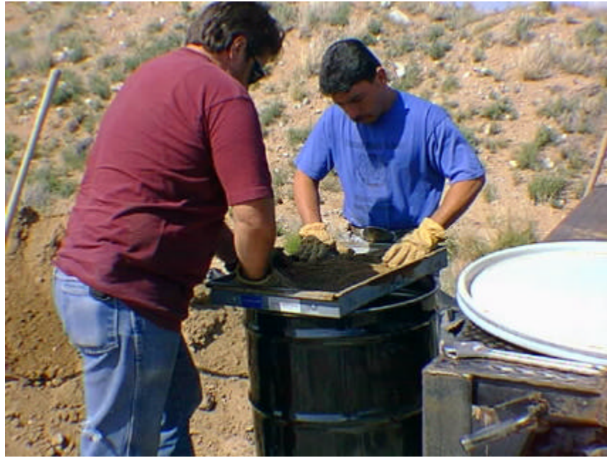
Figure C.2. Sieving the soil with a #8 screen.
