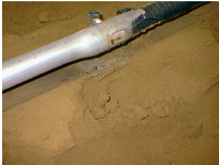
Figure 4.10. Radial expansion of the tube in Test 3.
