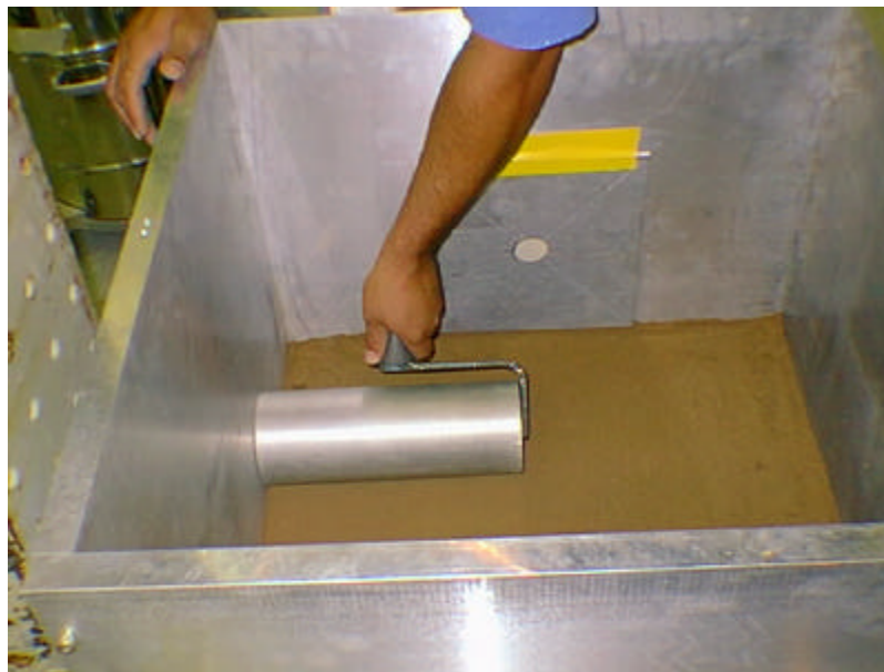
Figure C.5. Rolling the soil inside the explosive container.
