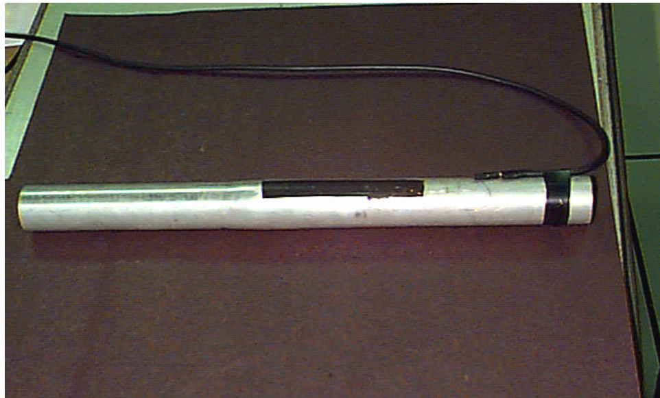
Figure D.4. Tube with the thin film carbon gage in place (electrical tape was placed over the gage).
