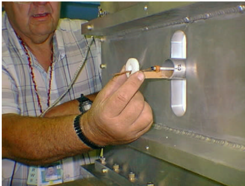
Figure B.2. Inserting an explosive charge into an assembled test fixture.
