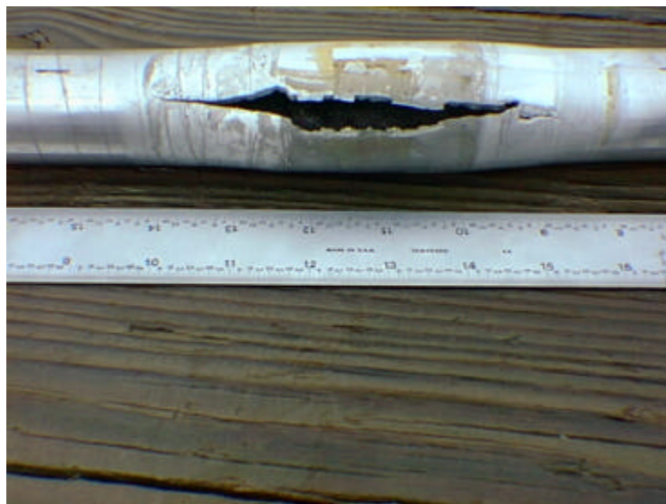
Figure 4.7. The center of the tube expanded by the action of the explosive charge.
